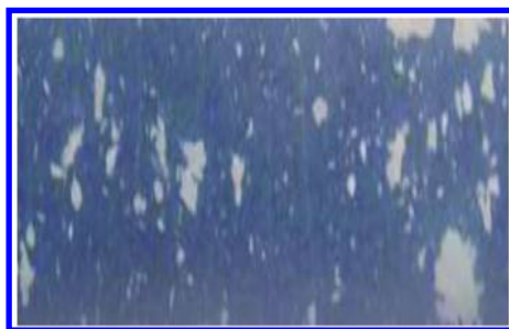
Figure 12. Water disintegration of TPSE/p-PVOH/copolyester 60/30/10 (Material 3), 60 seconds in water.
